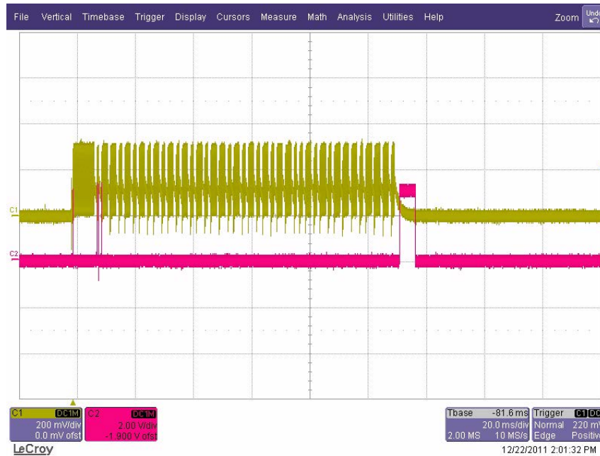
Figure 3-4. LF telegram used for MCU-direct mode example
