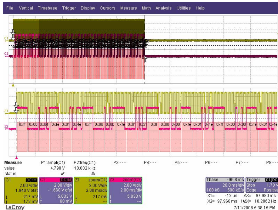
Figure 3-7. RF telegram received and decoded
