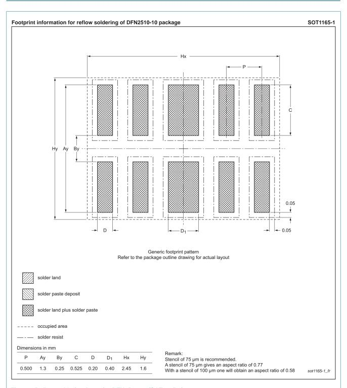
Fig 6. Reflow soldering footprint DFN2510-10 (SOT1165-1)
