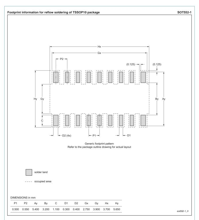
Fig 8. Reflow soldering footprint TSSOP10 (SOT552-1)
