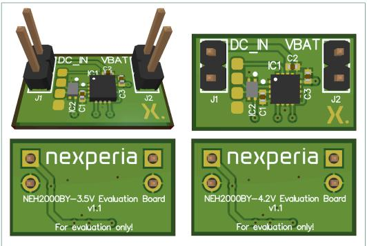
Fig. 1. NEH2000BY evaluation board 3D, top and bottom views
