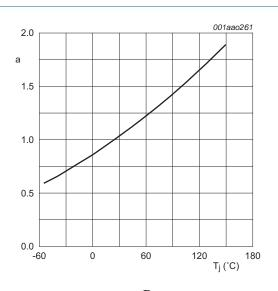
$a = \frac{R_{DSon}}{R_{DSon(25^{\circ}C)}}$
