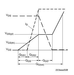
Fig 15. Gate charge waveform definitions
