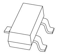
PBSS4230T 30 V, 2 A NPN low V<sub>CEsat</sub> (BISS) transistor
