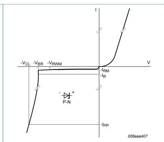
V-I characteristics for unidirectional ESD Fig. 4. protection diode
