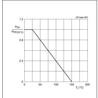
Fig.5 Relative variation of peak pulse power as a function of junction temperature; typical values.
