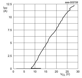
t<sub>p</sub> = 100 ns; Transmission Line Pulse (TLP)
