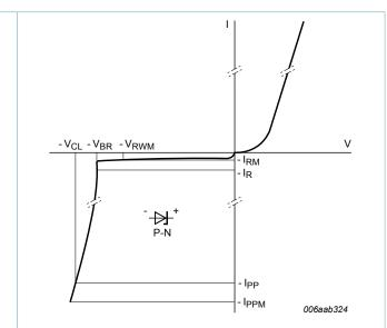
Fig. 4. V-I characteristics for a unidirectional ESD protection diode
