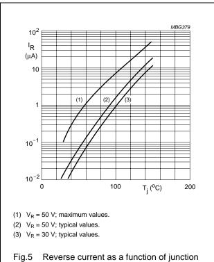
Fig.5 Reverse current as a function of junction temperature.
