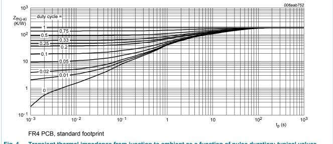
Transient thermal impedance from junction to ambient as a function of pulse duration; typical values Fig. 1.
