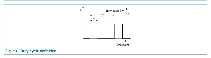
The current ratings for the typical waveforms are calculated according to the equations:  $I_{F(AV)} = I_M \times \delta$  with  $I_M$  defined as peak current,  $I_{RMS} = I_{F(AV)}$  at DC, and  $I_{RMS} = I_M \times \sqrt{\delta}$  with  $I_{RMS}$  defined as RMS current.
