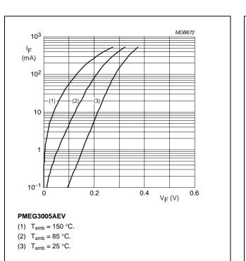
Fig.5 Forward current as a function of forward voltage; typical values.
