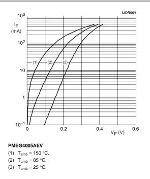
Fig.8 Forward current as a function of forward voltage; typical values.
