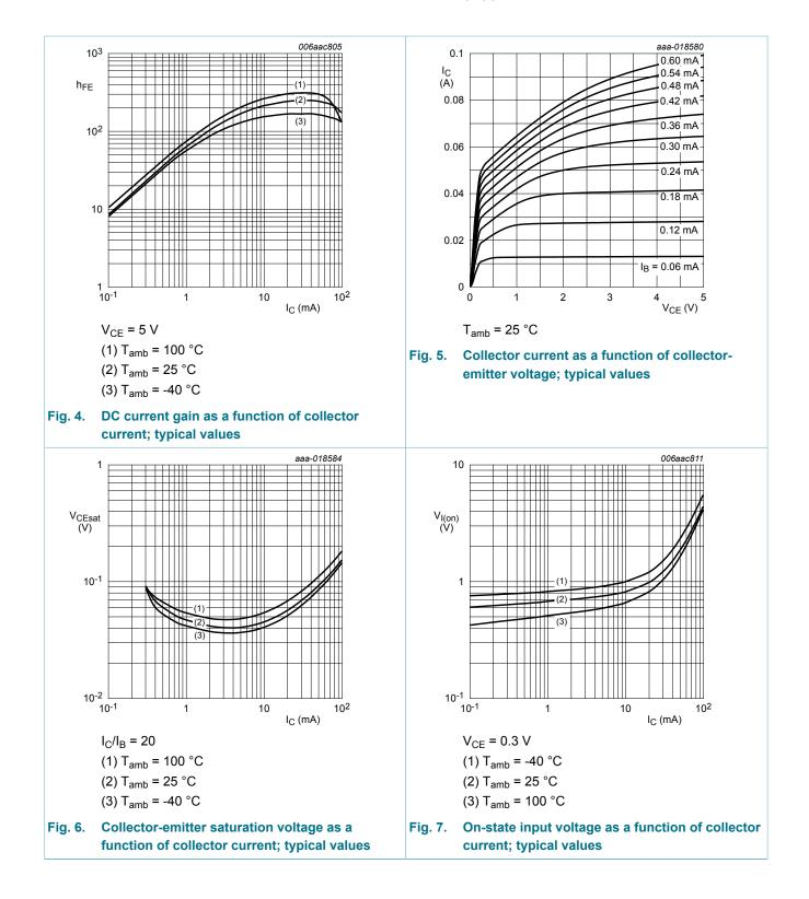
NPN/NPN resistor-equipped transistors; R1 = 2.2 k $\Omega$ , R2 = 47 k $\Omega$
