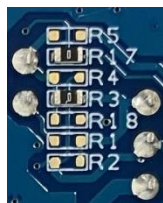
Fig. 4-3-1b I/O signal path around the PMIC and resistor lands
