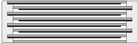
Extended metallized film design
