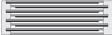
Extended metallized film design
