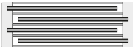
Extended double side metallized carrier film design
