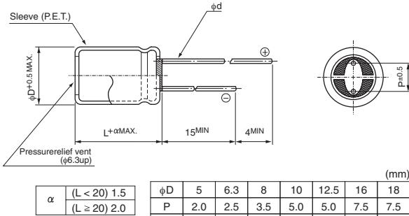
\*In case L > 25 for the φ12.5 dia. unit, lead dia. φd = 0.8mm
