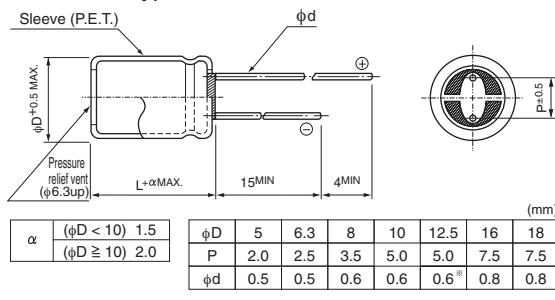
\*In case L > 25 for the φ12.5 dia. unit, lead dia.  $\phi d = 0.8$ mm.
