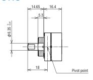
Unless otherwise specified, tolerance:  $\pm$  0.4 (Unit: mm)  $\langle$  **Accessories** $\rangle$
