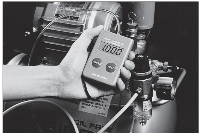
▲ Measurement of source pressure from a compressor.
