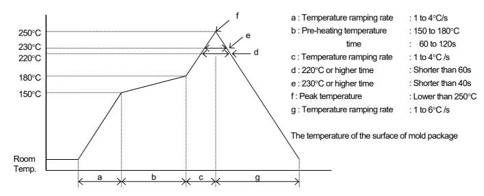
(NOTE1) Using reflow furnace with short wave infrared radiation heater such as halogen lamp Regarding temperature profile, please refer to those fo reflow furnace.
