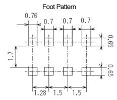
\*: Soldering is not required for dummy pattern.
