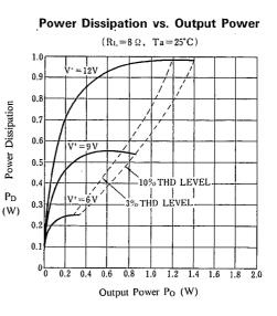
Power Dissipation vs. Output Power
