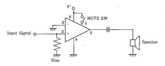
By this way, the bias circuit within IC, to be stopped and then, further for stopping motion of driver level, and at the output level. However, the input level alone is operating, so that a slight leakage of signal to the output pin through inside resistor to be occured. The leakage level is to be inverse proportion to load, therefore, it is necessary to check accordingly through the load condition.
