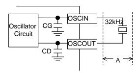
Typical externally-equipped element  $\begin{array}{c} \text{X'tal}: 32.768 \text{kHz} \\ \text{(R1=50k}\Omega \text{ typ)} \\ \text{(CL=6pF to 9pF)} \\ \text{Standard values of internal elements} \\ \text{CG,CD 10pF} \quad \text{typ} \end{array}$
