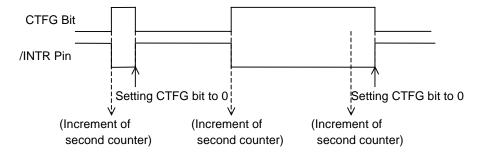
\*1), \*2) When the oscillation adjustment circuit is used, the interrupt cycle will fluctuate once per 20sec. as
