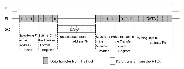
The reading and writing data transfer formats correspond to the settings in the transfer format register as shown in the table below.
