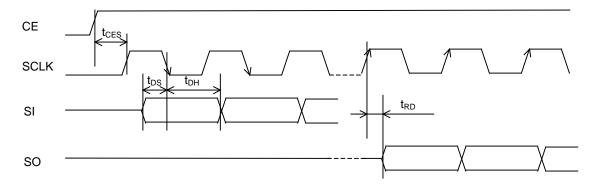
Conversely, when the SCLK pin is held high in the low to high transition of the CE pin, the models will select the timing with which the SO pin output is synchronized with the falling edge of the SCLK pin input, and the SI pin input is synchronized with the rising edge of the SCLK pin input, as illustrated in the timing chart below.
