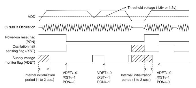
When the PON bit is set to 1 in the control register 2, the DEV, F6 to F0, WALE, DALE, /12·24, /CLEN2, TEST, CT2, CT1, CT0, VDSL, VDET, /CLEN1, CTFG, WAFG, and DAFG bits are reset to 0 in the oscillation adjustment register, the control register 1, and the control register 2. The PON bit is also set to 1 at power-on from 0v.
