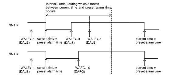
After setting WALE(DALW) to 0, Alarm registers is set to current time, and WALE(DALE) is set to 1, /INTR will be not driven to "L" immediately, /INTR will be driven to "L" at next alarm setting time.
