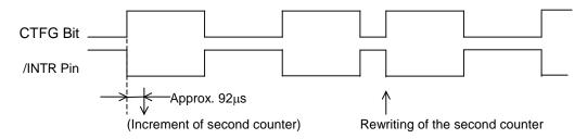
In the pulse mode, the increment of the second counter is delayed by approximately 92  $\mu$ s from the falling edge of clock pulses. Consequently, time readings immediately after the falling edge of clock pulses may appear to lag behind the time counts of the real-time clocks by approximately 1 second. Rewriting the second counter will reset the other time counters of less than 1 second, driving the /INTR pin low.
