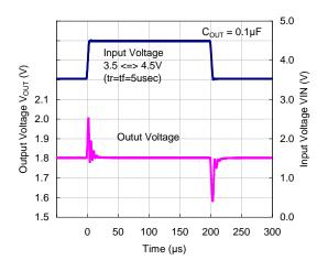
VR=3.3V,  $I_{OUT}$ =30mA,  $C_{OUT}$ =0.1 $\mu$ F
