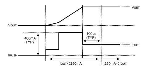
Likewise, on the thermal shutdown and the foldback characteristic, the inrush current preventing circuit works when the output voltage re-rises after the output voltage fall down to a guideline ( $V_{SET} \times 0.4$ ) or less.
