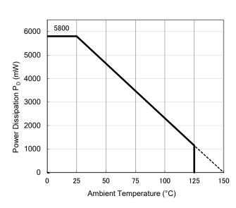
Power Dissipation vs. Ambient Temperature
