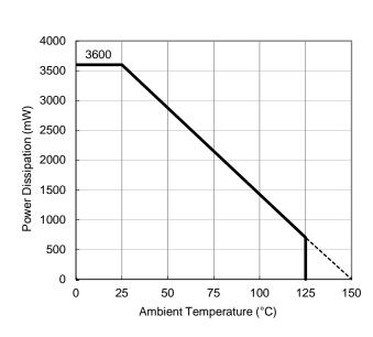
Power Dissipation vs. Ambient Temperature
