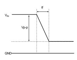
Prohibited Area of Fluctuation at Falling of  $V_{\text{IN}}$
