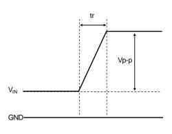
Prohibited Area of Fluctuation at Rising of  $V_{\text{IN}}$
