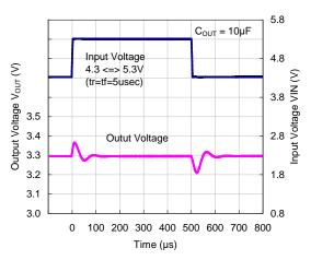
VR=5.0V,  $I_{OUT}$ =30mA,  $C_{OUT}$ =10 $\mu$ F
