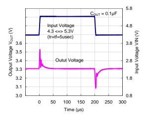
VR=5.0V,  $I_{OUT}$ =30mA,  $C_{OUT}$ =0.1 $\mu$ F
