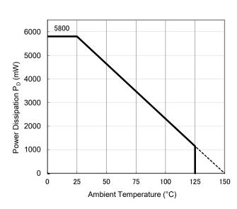
Power Dissipation vs. Ambient Temperature
