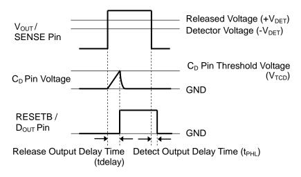
**Released Output Delay Timing Diagram**
