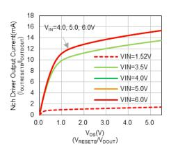
28) Nch. Driver Output Current vs. Input Voltage
