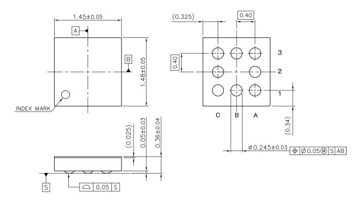
WLCSP-8-P1 Package Dimensions (Unit: mm)
