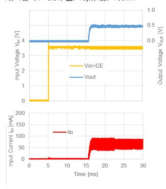
$V_{IN}$ =3.6V,  $V_{CE}$ =0V->3.6V,  $\triangle t$ =10 $\mu$ s,  $I_{OUT}$ =100mA
