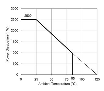
Power Dissipation vs. Ambient Temperature
