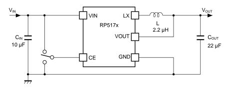
**Test Circuit of Typical Characteristics**
