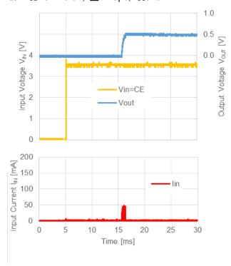
$V_{IN}=3.6V$ ,  $V_{CE}=0V->3.6V$ ,  $\Delta t=10\mu s$ ,  $I_{OUT}=0mA$
