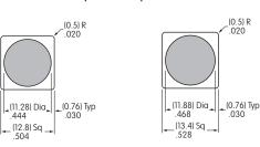
Film Insert Material and Thickness: Clear Polyester; 4 mil (100µ) maximum thickness
