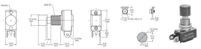
Dimension A: .185" (4.7mm) for NO model & .150" (3.8mm) for NC model. Dimension B Plunger Extension: .197" (5.0mm) for NO model & .161" (4.1mm) for NC model. Panel Thickness .193" (4.9mm)
