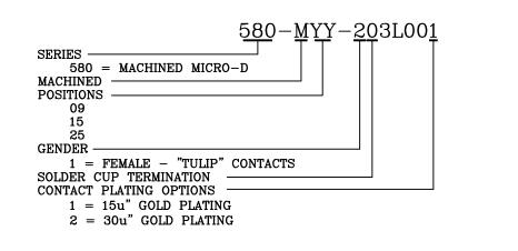
Rohs Compliant DO NOT SCALE FROM DRAWING UNITS = mm DRAWN: TOLERANCES SCALE: SHEET OF REV THESE DRAWINGS AND SPECIFICATIONS ARE .X .XX  $\pm 0.20 \\ \pm 0.10$ THE PROPERTY OF NorComp AND SHALL NOT J. KADEL NorComp NTS 2 1 BE REPRODUCED, COPIED OR USED AS THE  $\pm 0.05 \\ \pm 0.03$ .XXX DWG NO. DATE: BASIS FOR THE MANUFACTURE OR SALE OF .XXXX 580-MYY-203L001 05/12/2020 APPARATUS WITHOUT WRITTEN PERMISSION. ANGULAR ±1
