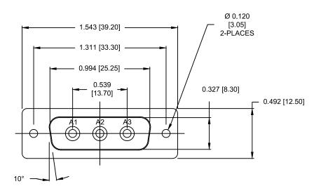
POWER CONTACT RESISTANCE:  $1.0 \text{ m}\Omega$  MAX. POWER CONTACT AMPERAGE: SEE P/N KEY
