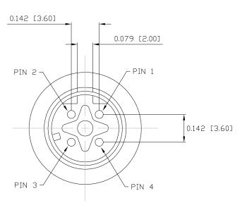
NOTE: MATERIAL HOUSING: PBT UL94V-0, BLACK CONTACT: BRASS NUT: BRASS □-RING: EPDM, BLACK SHELL: BRASS FINISH CONTACT: GOLD PLATED DVER 50u" NICKEL NICKEL PLATED NUT: SHELL: BRIGHT TIN PLATED ELECTRICAL RATED CURRENT: 4Α RATED VOLTAGE: 250V INSULATION RESISTANCE: 100 MOhms MIN. CONTACT RESISTANCE: 10 mOhms MAX. WATER PROOF: IP67 **ENVIRONMENT** OPERATION TEMPERATURE: -40°C T□ +85°C MAX WIRE AWG:
