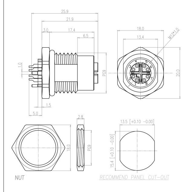
NOTE: MATERIAL HOUSING: PA66 UL94V-0, BLACK CONTACT: **BRASS** NUT: **BRASS** SHELL: **BRASS** □-RING: EPDM, BLACK ZINC ALLOY X-SHELL: **FINISH** CONTACT: GOLD 104" MIN. □VER 504" NICKEL NUT: NICKEL PLATED SHELL: NICKEL PLATED X-SHELL: NICKEL PLATED **ELECTRICAL** RATED CURRENT: 0.5A RATED VOLTAGE: 50VAC/60VDC INSULATION RESISTANCE: 100 MOhms MIN. CONTACT RESISTANCE: 10 mDhms MAX. WATER PROOF: IP67 **ENVIRONMENT OPERATION TEMPERATURE:** -40°C TD +85°C MAX WIRE AWG: 24
