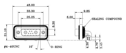
CONTACT Ø AT TERMINATION SIDE SIGNAL CONTACTS = Ø0.65 20 AMP = Ø2.80 40 AMP = Ø3.75
