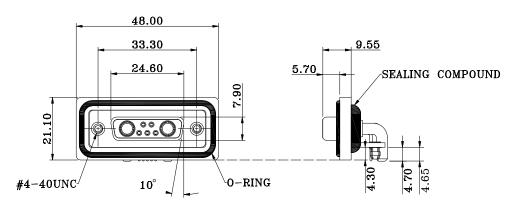
CONTACT Ø AT TERMINATION SIDE SIGNAL CONTACTS = Ø0.65 20 AMP = Ø2.80 40 AMP = Ø3.75
