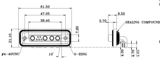
CONTACT Ø AT TERMINATION SIDE SIGNAL CONTACTS =  $\emptyset$ 0.65  $20 \text{ AMP} = \emptyset 2.80$  $40 \text{ AMP} = \emptyset 3.75$
