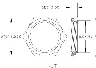
MATERIAL HOUSING: PBT UL94V-0, BLACK CONTACT: BRASS NUT: BRASS SHELL: BRASS D-RING: EPDM, BLACK FINISH CONTACT: GOLD PLATED, 10µ" Min. UNDER PLATE: NICKEL NUT: NICKEL PLATED SHELL: NICKEL PLATED M16\*1.50 ELECTRICAL RATED CURRENT: 250V RATED VOLTAGE: INSULATION RESISTANCE: 100MΩ MIN CONTACT RESISTANCE:  $10m\Omega$  MAX WATER PROOF: IP67/68 ENVIRONMENT OPERATION TEMPERATURE: -40°C ~ +85°C
