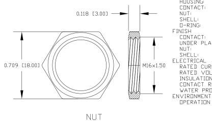
NOTE: MATERIAL HOUSING: PBT UL94V-0, BLACK CONTACT: BRASS BRASS NUT: SHELL: BRASS □-RING: EPDM, BLACK FINISH CONTACT: GOLD PLATED, 104" Min. UNDER PLATE: NICKEL NUT: NICKEL PLATED NICKEL PLATED SHELL: ELECTRICAL RATED CURRENT: 4Α 60V RATED VOLTAGE: INSULATION RESISTANCE: 100MΩ MIN CONTACT RESISTANCE:  $10m\Omega$  MAX WATER PROOF: IP67/68
