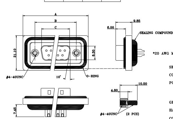
NOTE: MATERIAL HOUSING PBT UL94V-0, BLACK **FLANGE** PBT UL94V-0, BLACK CONTACT BRASS, PLATING P/N KEY BELOW SHELL STEEL, NICKEL SILICONE O-RING **EPOXY** SEALING COMPOUND **HARDWARE** BRASS; NICKEL PLATED **ELECTRICAL** RATED CURRENT 5A 1000 VAC 1 MIN VOLTAGE INSULATOR RESISTANCE 5 GOhms MIN. CONTACT RESISTANCE 10 m0hms MAX. WATER PROOF IP67 ENVIRONMENT
