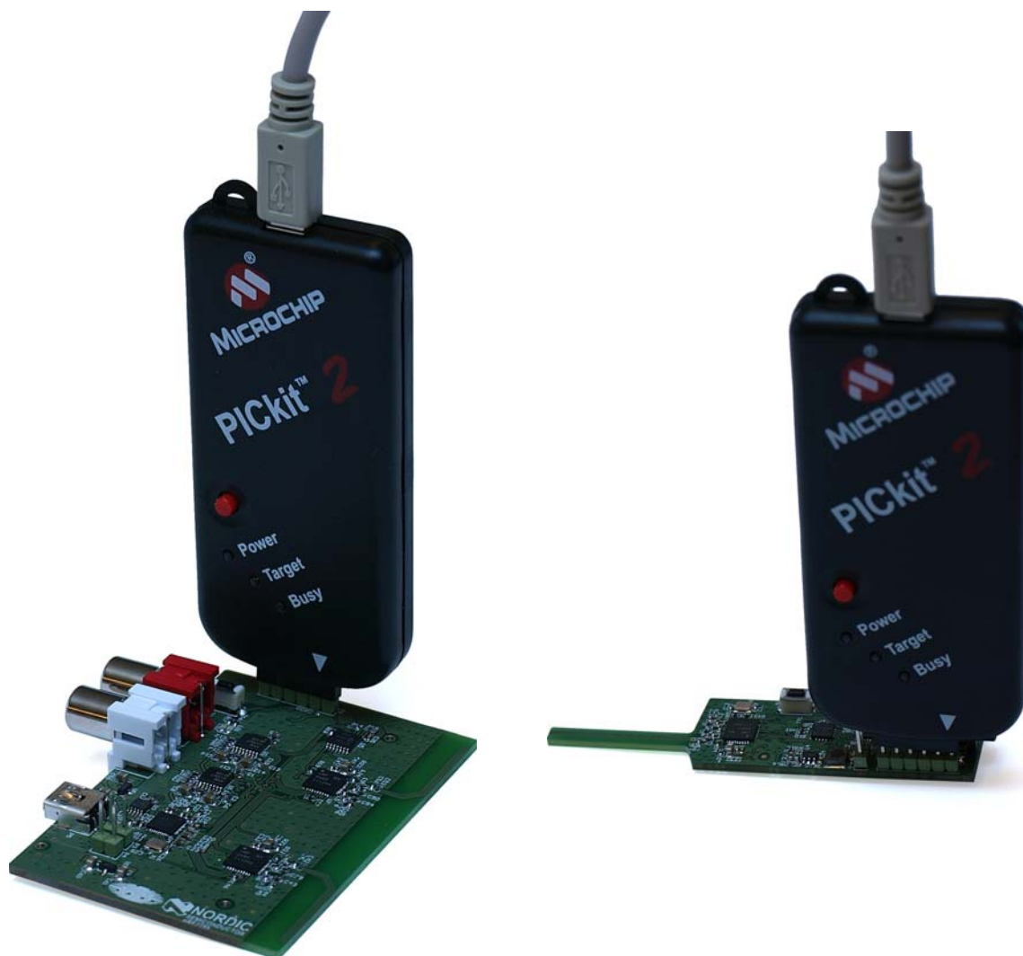
Figure 3. Receiver board and microphone setup with PICkit2™
