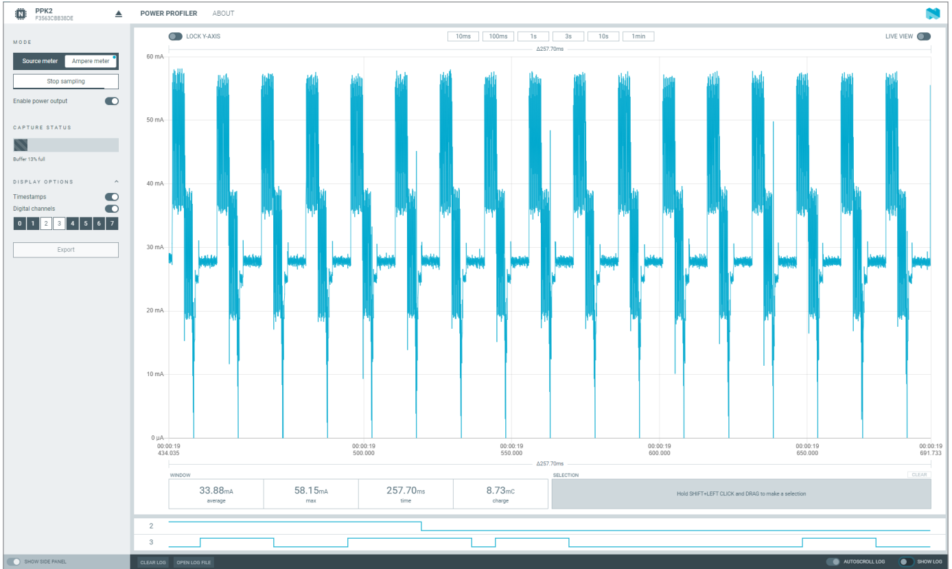
Screenshot of the Power Profiler app running on the nRF9160 DK in ampere meter mode.
