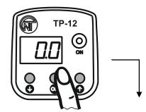
Press OK pushbutton to enter parameter, thus the display shows factory parameter setting in (D.D) flashing mode
