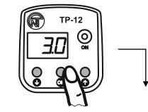
Press **OK** pushbutton to enter parameter, thus the display shows the factory parameters setting in  $(\exists . D)$  flashing mode
