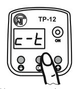
Via Or pushbutton change parameter value within -5.0 to +5.0 °C with increment size of 0.1 °C
