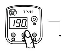
Press **OK** pushbutton to enter parameter, thus the display shows factory parameter setting in (**ISD.**) flashing mode
