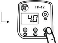
Via O or pushbutton change parameter value within 0.1 to 30 °C with increment size of 0.1 °C
