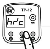
Hold **OK** pushbutton pressed for 3 seconds until the display shows «hrc» menu parameter
