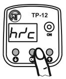
Hold **OK** pushbutton for 3 seconds until the display shows «hr/c» menu parameter
