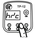
Hold **OK** pushbutton pressed for 3 seconds until the display shows «hr/c» menu parameter
