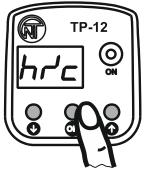
Hold **OK** pushbutton pressed for 3 seconds until the display shows «hr/c » menu parameter
