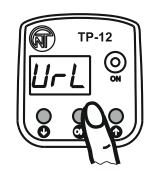
Press **OK** pushbutton to save changes, thus the display shows «*Ur-L*» menu parameter (in case of holding **OK** pushbutton pressed for 3 seconds, one exits settings menu without saving and the device will operate in normal mode).
