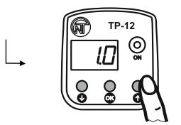
Via Or Or pushbutton change parameter value within 0 to 10 minutes with increment size of 1 minute. When setting 1 minute the device turns on / off the load in 1 minute.
