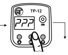
Press **OK** pushbutton to enter parameter, thus the display shows three question marks in flashing mode
