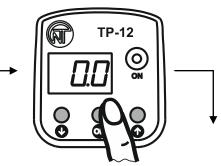
Press **OK** pushbutton to enter parameter, thus the display shows factory parameter setting in (**D.D**) flashing mode
