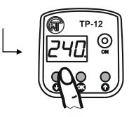
Via  $\bigcirc$  or  $\bigcirc$  pushbutton change parameter value within 230 to 290 V with increment size of 5 V
