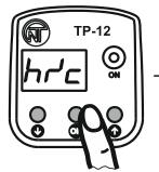
Hold **OK** pushbutton pressed for 3 seconds until the display shows **whrlc** menu parameter
