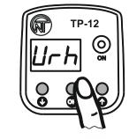
Press **OK** pushbutton to save changes, thus the display shows «Urh» menu parameter (in case of holding **OK** pushbutton pressed for 3 seconds, one exits settings menu without saving and the device will operate in normal mode). To exit menu hold **OK** pushbutton pressed for 3 seconds
