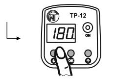
Via **O** or **O** pushbutton change parameter value within 120 to 210 V with increment size 5 V
