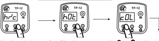
Hold **OK** pushbutton for 3 seconds until the display shows «hr/c» menu parameter
