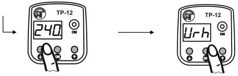
Via or pushbutton change parameter value within 230 to 290 V with increment size of 5 V
