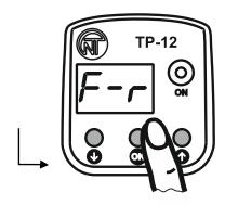
Press OK pushbutton to reset all configurable parameters to factory settings, thus the display shows «F-r» menu parameter (in case of holding OK pushbutton pressed for 3 seconds, one exits reset settings menu to factory settings and the device will operate in normal mode).
