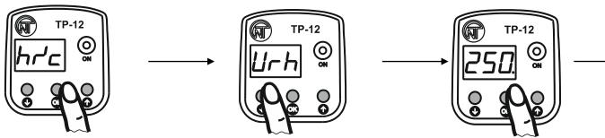
Hold **OK** pushbutton pressed for 3 seconds until the display shows «hr'c» menu parameter
