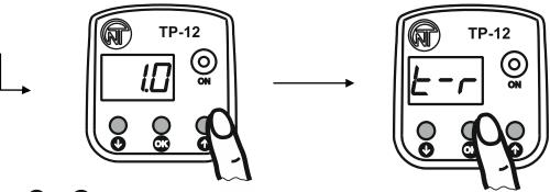
Via or pushbutton change parameter value within 0 to 10 minutes with increment size of 1 minute. When setting 1 minute the device turns on / off the load in 1 minute.
