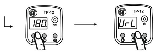
Via ♥ or ♠ pushbutton change parameter value within 120 to 210 V with increment size 5 V
