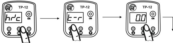
Hold **OK** pushbutton pressed for 3 seconds until the display shows «hr/c» menu parameter
