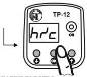
Press OK pushbutton to save changes, thus the display shows «hr'c» menu parameter (in case of holding OK pushbutton for 3 seconds, one exits the setting menu without saving and the device will operate in normal mode).
