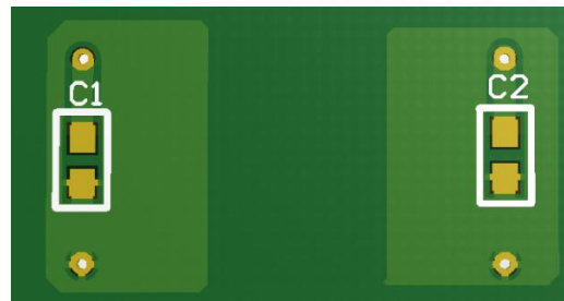
Figure 6.3 Recommended PCB Layout — Bottom Layer
