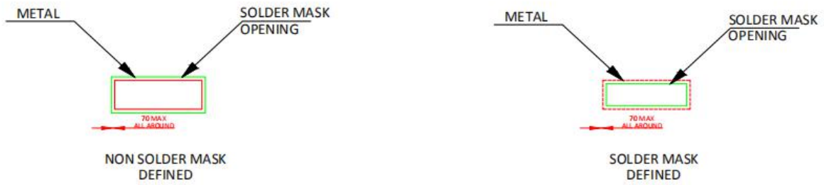
Figure 9.2 SOW8 Package Board Layout Example
