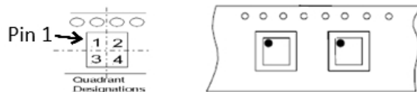
Figure 12.5 Quadrant Designation for Pin1 Orientation in Tape
