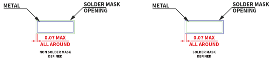
Figure 9.4 SOW8 Package Board Layout Example
