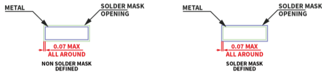
Figure 9.6 SOP16(300mil)/SOW16 Package Board Layout Example
