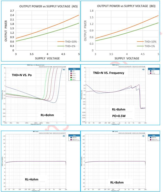
In the following characteristic curves, T=25  $^{\circ}$ C (unless conditions are specified).
